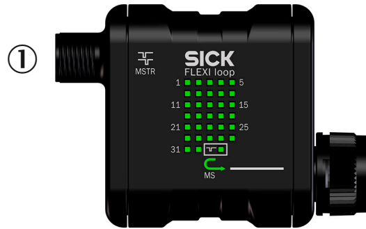
Figure 46: Connections of the MSTR1 Flexi Loop accessory
